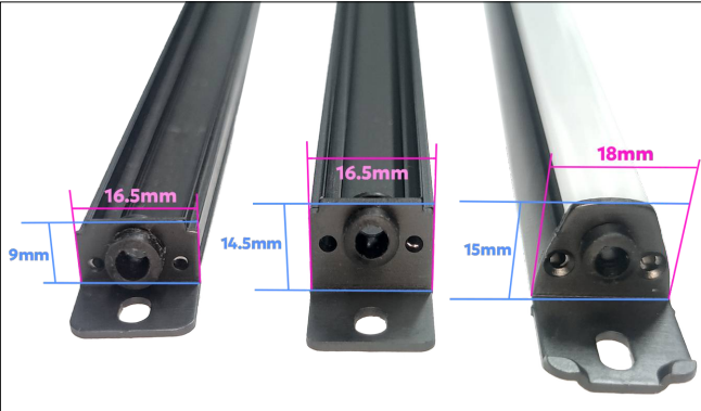
Size comparison of Aluminum light strips L: Classic M: Classic + Mount Rails R: Stealth
